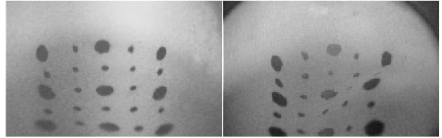
Figure 3: Camera view of membrane: (a) undeformed (b) in contact with an object.
