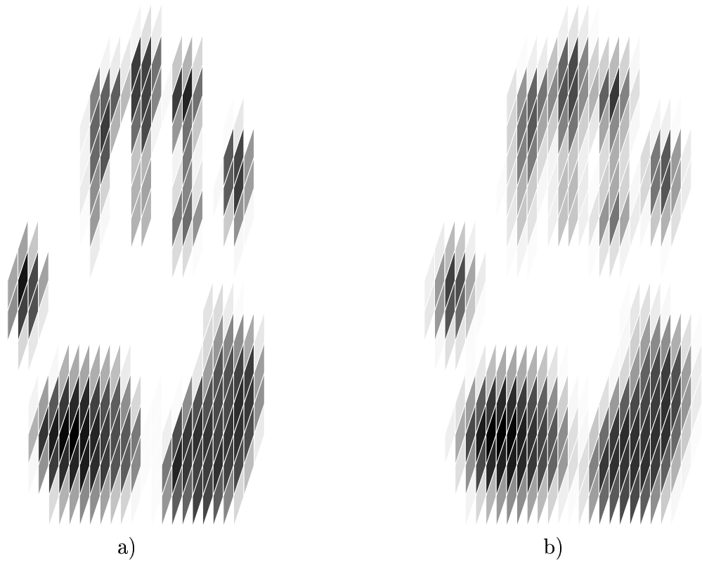
Figure 3.6: Unsmoothed a) and diffused b) proximity images of a flattened hand with the fingers squeezed against one another rather than spread out. Note that smoothed proximities of pixels near the center of each contact are more even but proximity has also bled outward around contact edges, as is especially noticeable for the thumb contact.
