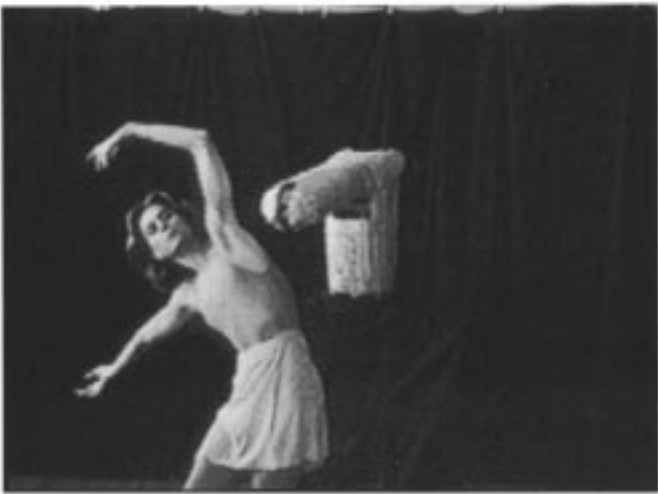
Fig. 2. Ballerina dancing with a robot manipulator. As with two human partners, the whole dance is pre-rehearsed, but their actual positions at any given moment differ from one "performance" to the other. Since the robot's sensitive skin allows it to continuously sense the ballerina, she can trust her partner enough to turn her back to it and expect a "correct," collision free reaction. (V. Lumelsky, Robotics Laboratory, University of Wisconsin-Madison.)
