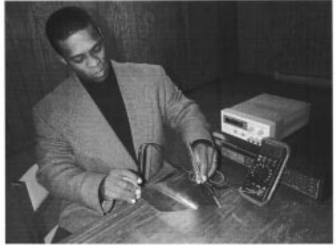
Fig. 8. \text{Cu}_x\text{S} transparent metal film deposited on flexible view foil. (Courtesy of BIT's, Inc.)
