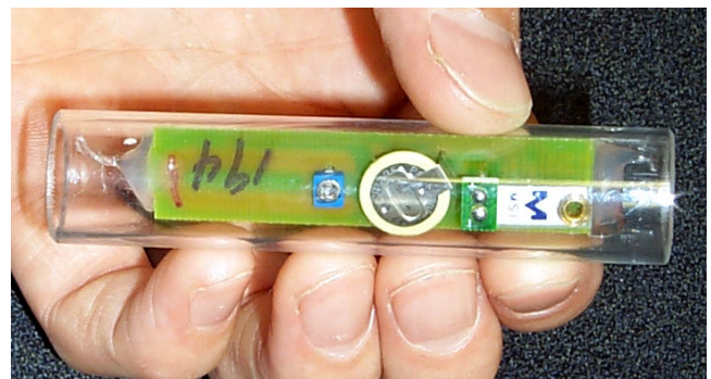
Figure 5: Low cost “jerk” sensor to instrument large crowd
