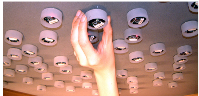
Figure 7: 100 Pushpin nodes pushed into their substrate
