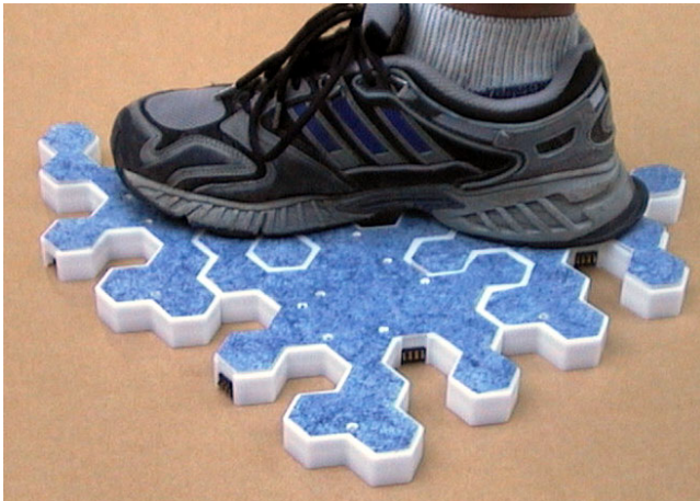
Figure 9: A few assembled Z-Tiles under test
