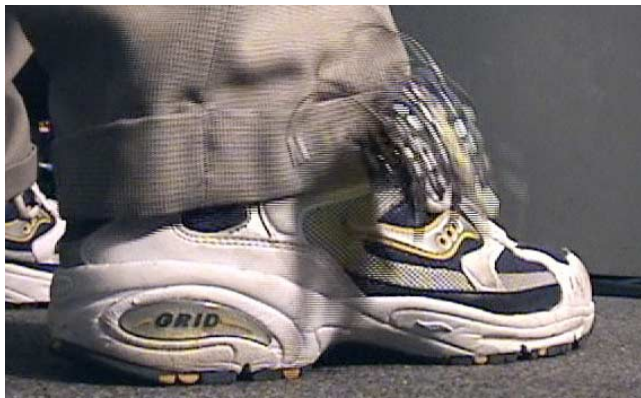
Figure 7: An Active Parasitic Mobility Node, detecting a proximate host (top) then launching and grappling onto their cuff (bottom).
