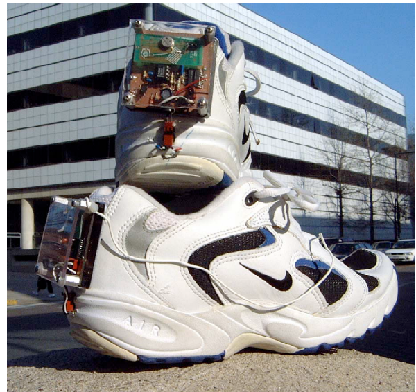
Figure 5: A pair of sneakers equipped with piezoelectric power-generating insoles and self-powered transmitter.
