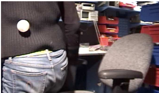
Figure 8: A sticky Passive Parasitic Mobility Node coated with silicone adhesive, having just transferred to the user's sweater from the chair back.
