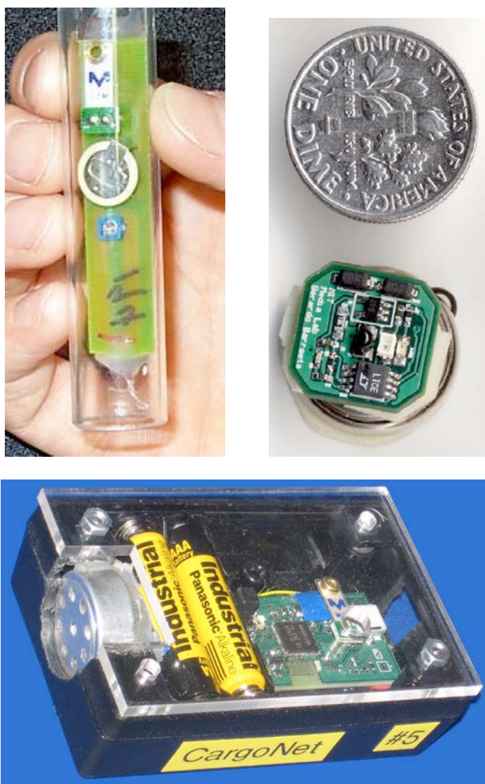
Figure 3-5. An ultra low-cost wireless motion sensor for crowd interaction (top left), quasi-passive optical wakeup tag (top right), and a CargoNet Active RFID Sensor Tag (bottom).
