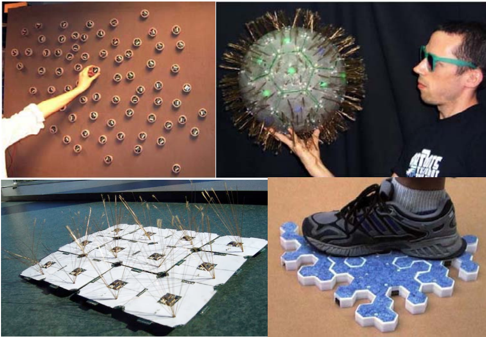
Figure 3-9. Several Dense Sensor Networks - the PushPin Computer (top left), the Tribble (top right), a sensor network “skin” with elements fabricated on flex substrate (bottom left), and a few of the Z-Tiles interactive floor (bottom right) pursued in collaboration with the University of Limerick
