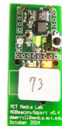
Fig. 2 A demo placard with a "Squirt" (a compact IR tagging beacon) at lower right
