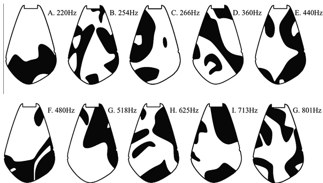
Fig. 8. Eigenmode gradient maximum values. For each mode, the black areas are sensors candidates – the one third of the surface area with the highest absolute value of gradient.
