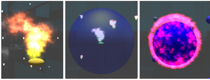
Fig. 3. Thermostats are represented by colored flames (left). An anomaly between the setpoint and measured temperature is indicated by a pulsating sphere (center) and an alternate visualization (right) shows the magnitude of the discrepancy.
