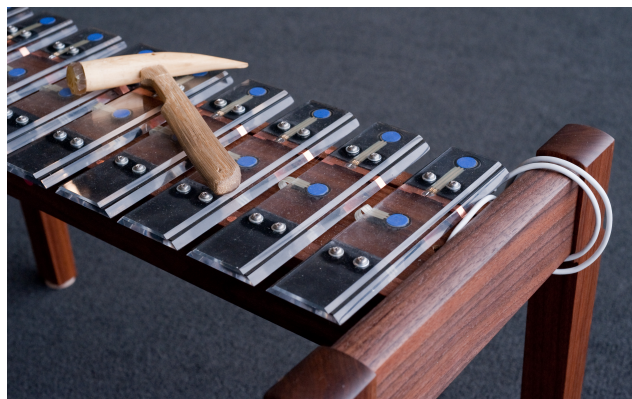
Figure 2: Pemade with rubber tipped panggul . Two FSRs between acrylic detect central strike and edge damping.
