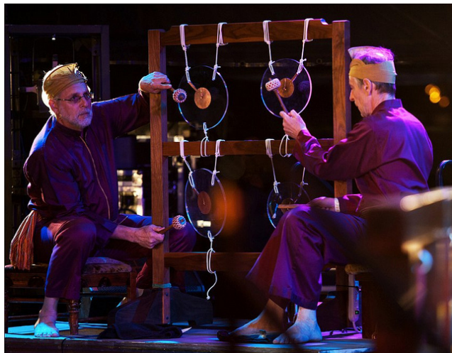
Figure 4: Gamelan Elektrika gongs being performed by Mark Stewart and Jacques Weissgerber. Rear mounted piezos discs are used to detect the strike while the gold discs in the center provide dampening through capacitive sensing. Photo by Kevin Yatarola
