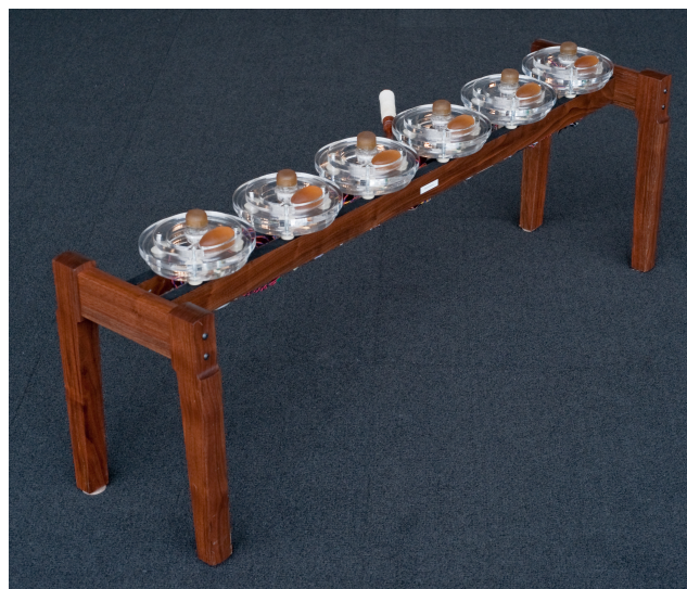
Figure 3: One half of the reong holding six pots. The center is a free-standing rod with piezo films and FSRs placed underneath used to implement byongs . The small pads on the right are the chucks .
