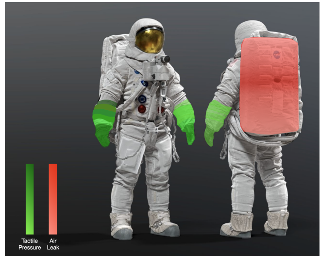
Figure 2. Illustration of SpaceTouch Graphical User Interface (GUI) for real-time physical interaction visualization and safety assessment.
