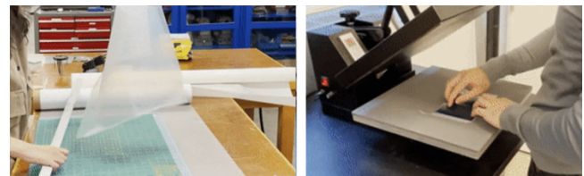
Figure 9: Students inspired by PneuBots making their own inflatable designs a) cutting a PVC film b) using a heat press to join two layers of PVC films.
