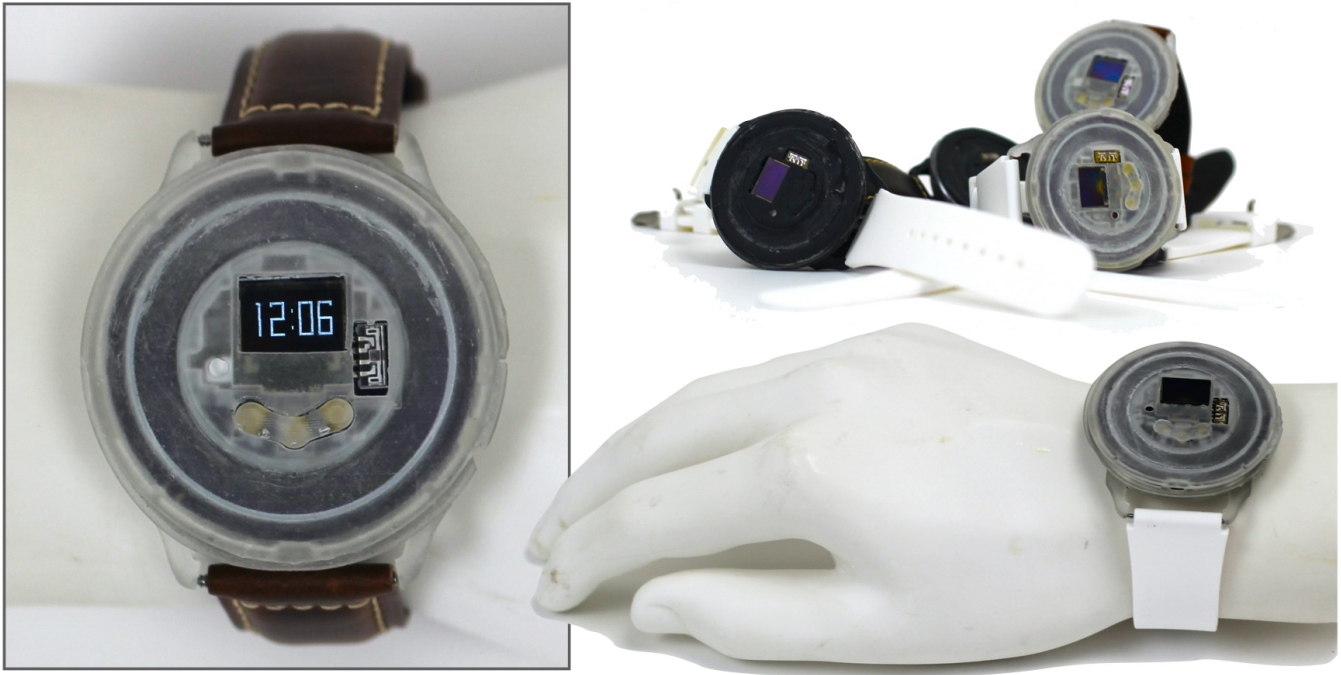
Figure 1: The custom 'Equinox' watch can notify the user, monitor ambient light levels, and collect time estimates, duration estimates, or experience sampling survey data all day long. In our initial test, we ask users to guess the time in order to check the time.
