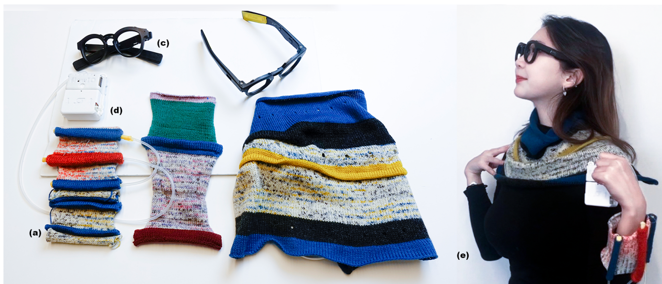
Figure 1: (a) NugiTex arm warmers constructed of tubular soft materials that constrict when actuated (b) Neck warmer with embedded circular soft material (c) AirSpec ® , an environmental sensing device for to capture ambient temperature and humidity (d) FlowIO [12], a development platform for soft robots and programmable materials for controlling the airflow of NugiTex. (e) A user wearing NugiTex, AirSpec, and FlowIO.
