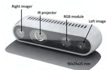
**Fig. 14** Intel RealSense D435i stereo and RGB integrated depth camera.
