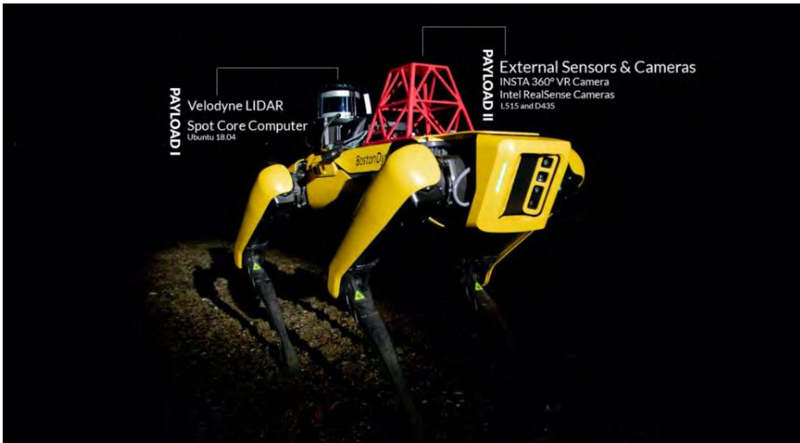
**Fig. 16 Boston Dynamics Spot robot with first payloads mounted: Velodyne LiDAR puck, SpotCORE onboard computer, and custom payload tower (red).**
