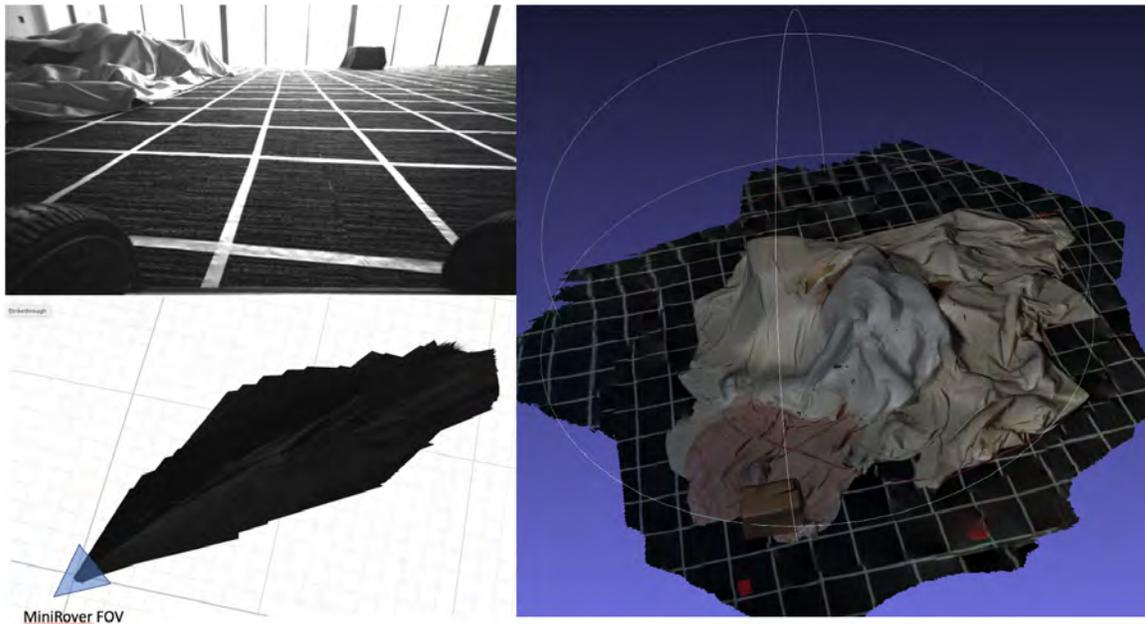
**Fig. 15** Depth-camera views. **Top-Left:** Intel RealSense D435i stereo and RGB integrated depth camera snapshot from a complete traverse - captured using SLAMCore software. **Bottom-Left:** Intel RealSense D435i stereo and RGB integrated depth camera single waypoint depth-data capture - captured using RealSense Viewer. **Right:** Lumentum VCSEL structured light and RGB integrated depth camera for full environment capture - rendered as obj file with iPhone integrated software.
