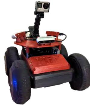
**Fig. 10** RoverRobotics mini rover with custom payload mount for three Intel RealSense D435i cameras (forward facing and two rear facing cameras positions 45° from backward). An additional GoPro camera was mounted on the rover.
