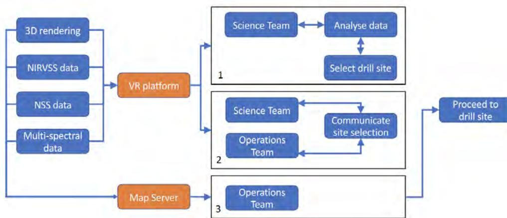
**Fig. 9 Task oriented Concept of Operations for drill site selection.**
