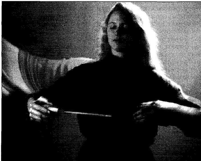
[8] A "conductor" wielding a Digital Baton works with acceleration, light, and finger or hand pressure. The precise position of the baton tip in two-dimensional space is tracked by an infrared light-emitting diode [LED] and a photosensor. The visible LED on the tip both gives directional feedback to the conductor and brightens in response to pressure on the baton. Beats and large gestures in all directions are monitored with the accelerometers. Five force-sensing resistors encased in the baton's urethane skin react to pressure from individual fingers or the palm of the hand.
