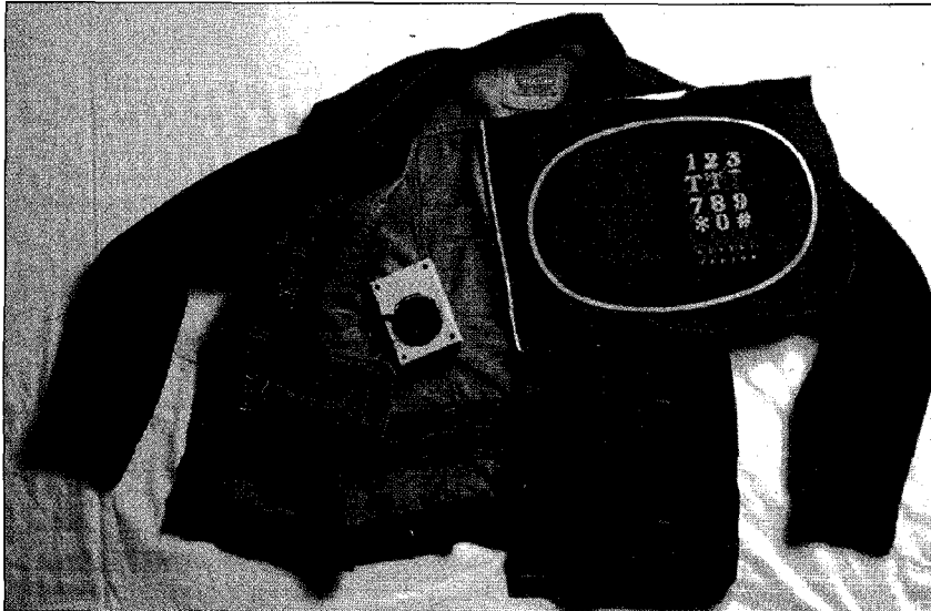
[12] Slip into a comfortable synthesizer in the guise of this jacket stitched with conductive thread. The boat-shaped board [left] houses a single-chip synthesizer. A MIDI controller with 12 touch-sensitive "keys" lines the swatch that will be stitched on the jacket.
