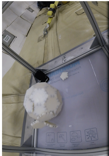
Fig. 12 An example of unintentional magnetic interaction between non-bonding faces of the tiles. The remaining assembly (partial buckyball) was manually assembled to test hole-filling in this particular parabola scenario.
