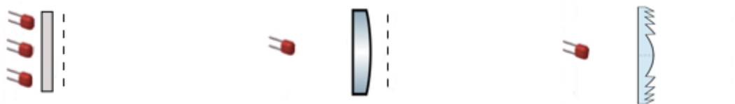
Figure 9. The back-illumination of the coded mask. Left: an array of LEDs illuminate a diffusor. Center: the light of a single LED, placed in the focus of a condenser lens, is beamed through the mask. Right: the condenser lens is replaced by a (plastic) Fresnel lens. The distance between the mask and the Fresnel lens should be larger than the depth-of-field of the optical system, to avoid a circular pattern to be projected on the pixel sensor, superimposed on the mask pattern.
