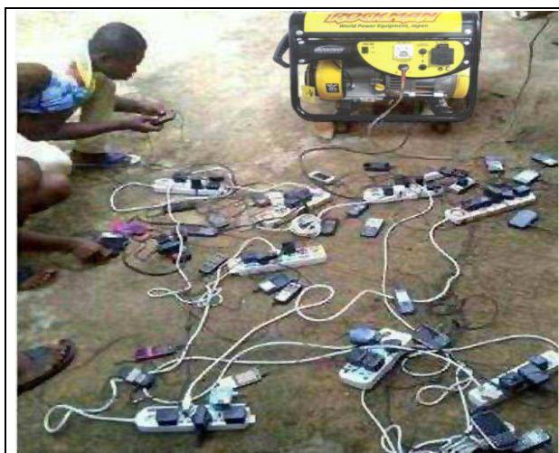
Figure 1. An ad hoc nano-grid use to charge cell phones from an electrical generator.
