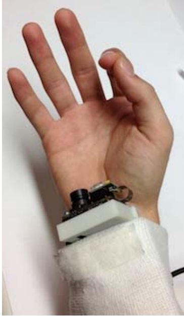
Fig. 2. The camera and microphone on the user's wrist, user performing the index pinch microgesture.
