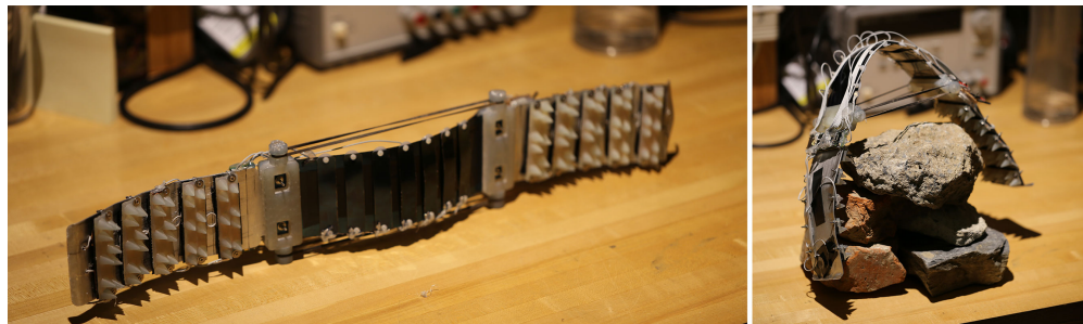
Fig. 8 Single node Grapple with a n=1 bistable elements and flat end effectors
