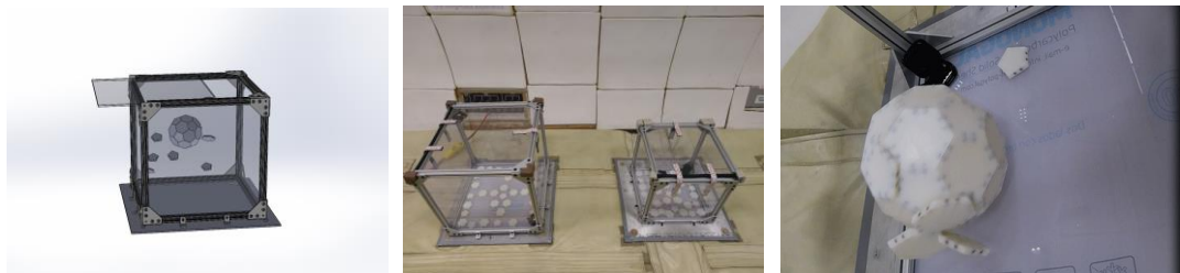
Figure 6. Experimental test apparatus for microgravity flight (Left/Center), assembly behavior example (Right).
