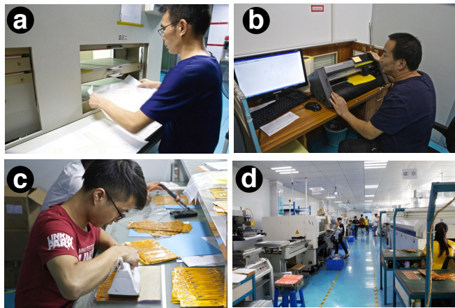
Fig. 3. Pictures of selected manufacturing steps in the factory. a) The technician is placing the flexible PCB in a heat press to laminate the coverlay. b) Vinyl cutting the wax paper for creating air pouches c) Manual alignment of the coverlay followed by temporary attachment of the coverlay with a cloth iron. d) The SMT assembly line used to assemble the robots.
