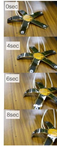
Fig. 8. Snapshots of the air actuated robot moving.
