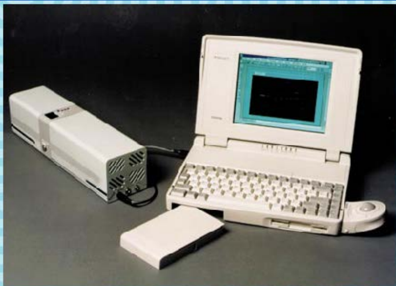
A laptop computer using a fuel cell power source can operate for up to 20 hours on a single charge of fuel. (Courtesy: Ballard Power Systems)
