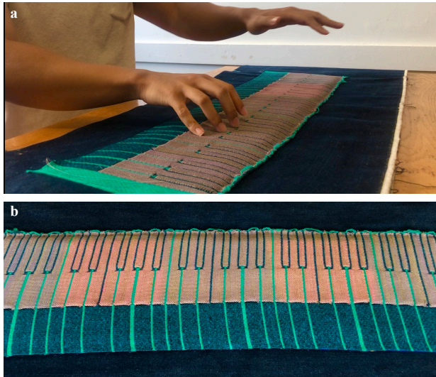
Figure 5: a) Modes of interaction: one hand's hovering and the other playing keys, and b) thermochromic color change in action for proximity field sensing marker (from grey to pink).
