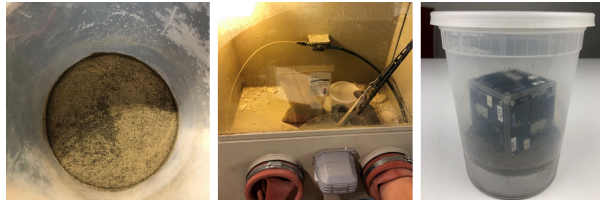
Figure 22: Water detection test with LMS-1.
