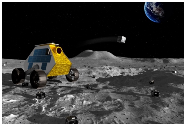
Figure 25: LunarWSN nodes deployed from a rover.
