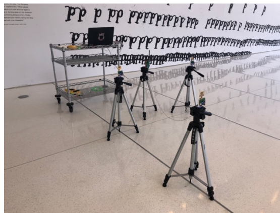
Figure 12: Ranging anchors and central station set up for the localization test.
