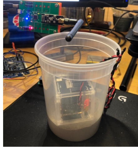
Figure 19: Water detection test setup with sands.
