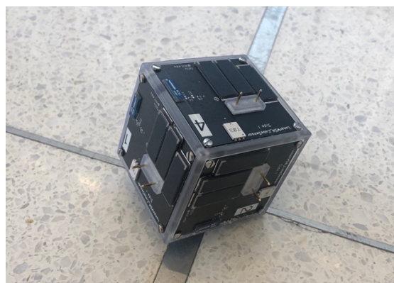
Figure 13: Node is put atop a floor joint
