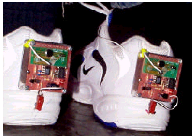
Figure 9: Piezo-powered shoes w. mounted electronics
