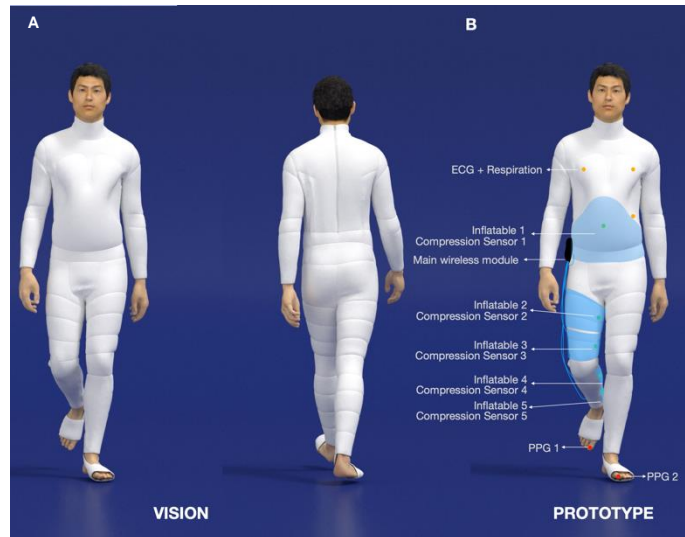
Fig.5: a) PS-Suit concept and b) illustration of our recent prototype flown in a parabolic flight, showing all the main component of the system (inflatable chambers, fabric compression sensors, physiological sensors, and main wireless module).
