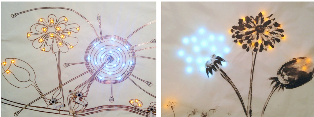
Figure 3. Circuitry (left) and painting overlay (right) of Dandelion painting.
