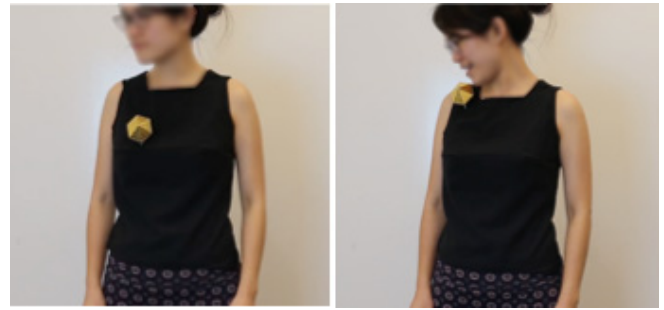
Figure 13. Interactive moving jewelry. Robotic brooch moves to become a shoulder microphone speaker when wearer receives phone call.
