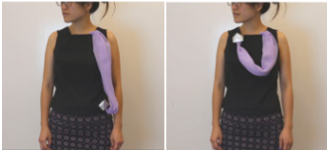
Figure 12. Shape changing fabric. Robot self-attaches to fabric ends shifts to become a scarf according to temperature change.
