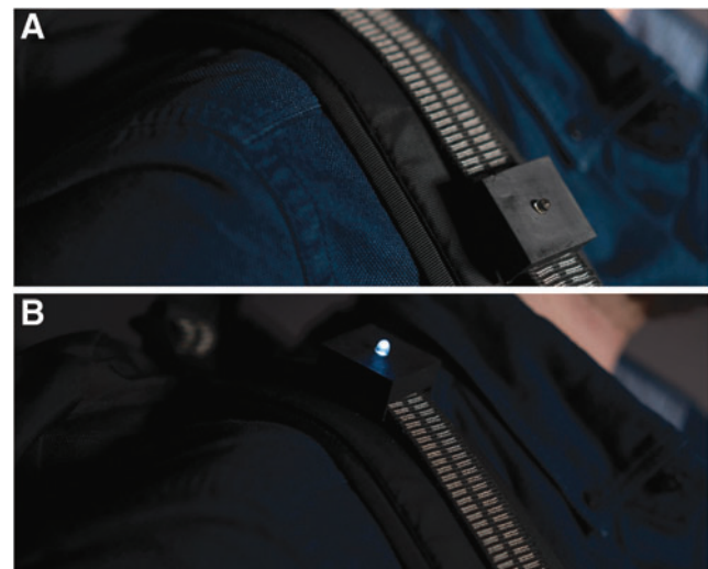
FIG. 13. Customized belt rheostat sewn onto a backpack with a 3D-printed enclosure that covers the buckle, and a voltage divider circuit that changes the brightness of an LED; (A) low brightness, (B) high brightness. LED, light-emitting diode.
