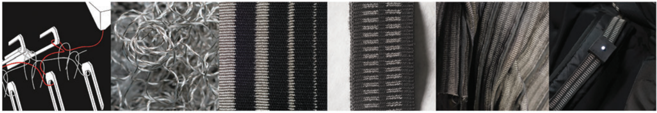
FIG. 1. Left to right : interlocking structure with two-bed machine knitting; close view of conductive yarn; conductivity test knit sample with varying width; belt rheostat; mass produced knitted belt rheostat; belt light application.
