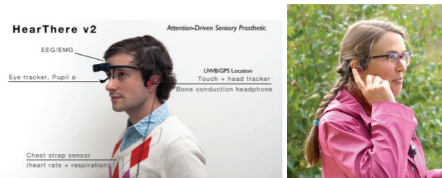
Figure 6: Attention-Driven Auditory Prosthetic – early research prototype (left) and subsequent Tidmarsh-fielded version (right)
