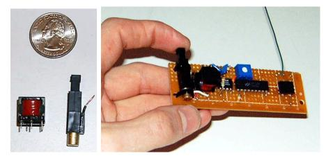
**Fig. 2.** Critical components (left – not including US quarter) and operational prototype board (right) for self-powered wireless ID pushbutton transmitter of Fig. 1
