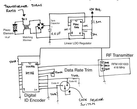
Fig. 1. Schematic diagram of self-powered pushbutton electronics
