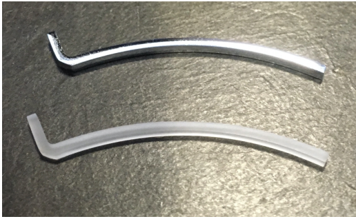
Fig. 13. PMMA Light Pipe: Chrome-Plated (Top) and Non-Plated (Bottom)
