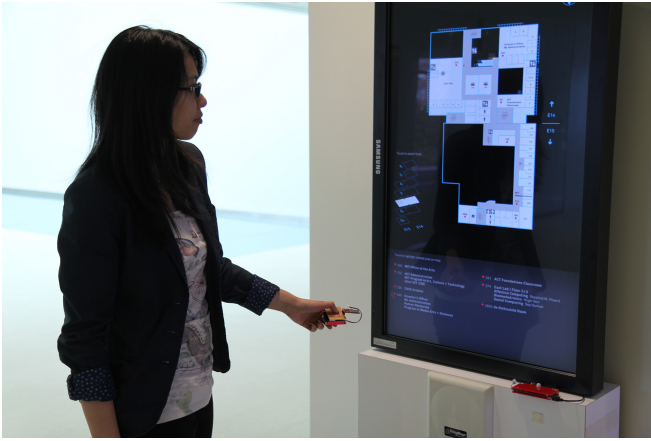
Fig. 5. An example usage scenario with a display kiosk. The user holds the EMI Spy at its grounded battery, hence captures the electromagnetic interference from proximate electronic devices via its sensing electrode. These noise signatures are then used to uniquely identify the devices and detect gestures such as pointing at a distance and touch in real-time.
