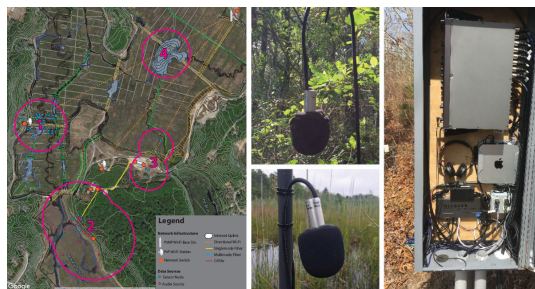
Figure 1. Sensors, microphones, and cameras are deployed in four regions of interest at Tidmarsh. Custom sensors have been specially designed to withstand wetland conditions year-round.
