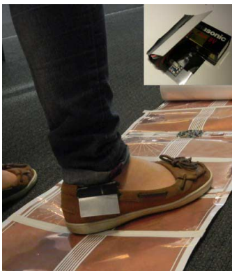
Figure 15. Illustration of transmitting/receiving into the floor – from clip on shoe to floor.
