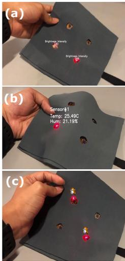
**Figure 8:** Three different visualizations of the LEDs when turned on. a) shows brightness intensity, b) the sensor streams, and c) a mole game.
