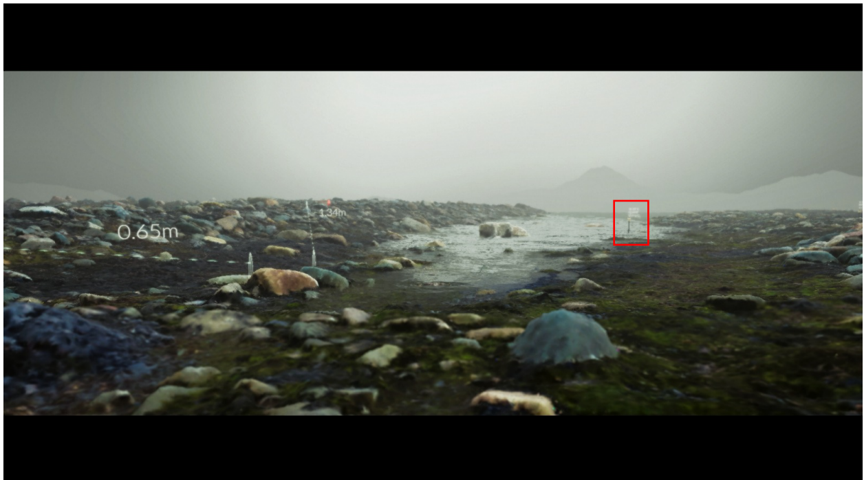
Figure 14: Preliminary virtual environment in Unity of Site 1, riverbed. Data was collected using the drone. Red box highlights the sensor node, white dashed lines to cones with hovering numbers show measurement tool capabilities.
