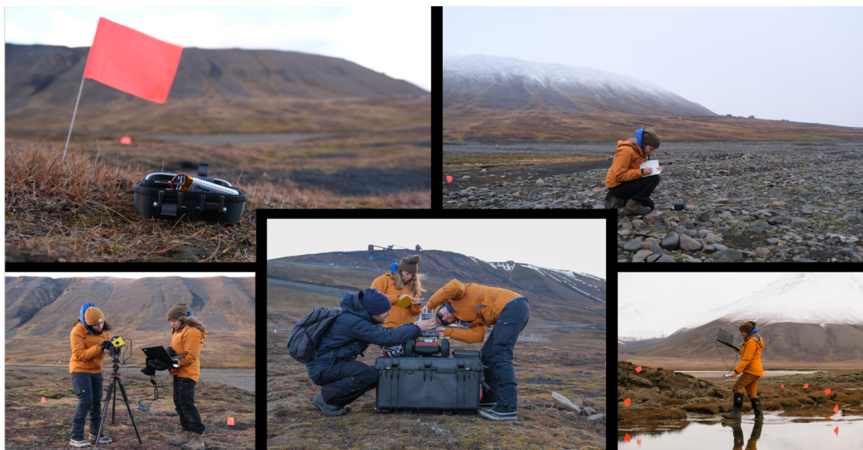
Figure 8: Clockwise from top left: Arduino environmental sensor in custom hard-shell case, C. Paige collecting field notes, C. Paige collecting data using the Microsoft Azure Kinect, C. Paige, S. Auffinger and J. Todd preparing a mini rover with the Microsoft Azure Kinect mounted on a custom payload tower for data collection, C. Paige and J. Todd collecting data using a Velodyne puck on a custom 360-degree rotational mount (collection for a separate project, Ward et al., at ICES 2023).
