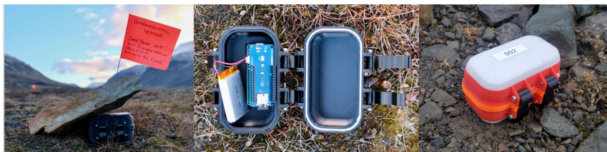
Figure 9: The Arduino Nano 33 BLE Sense environmental sensor is contained in a custom weatherproof housing for data collection. Left – sensor is flagged and housing is closed and weighted for overnight data collection, Middle – shows housing opened for researcher-on-site data collection with Li-Ion battery connected and Right shows custom weatherproof housing.
