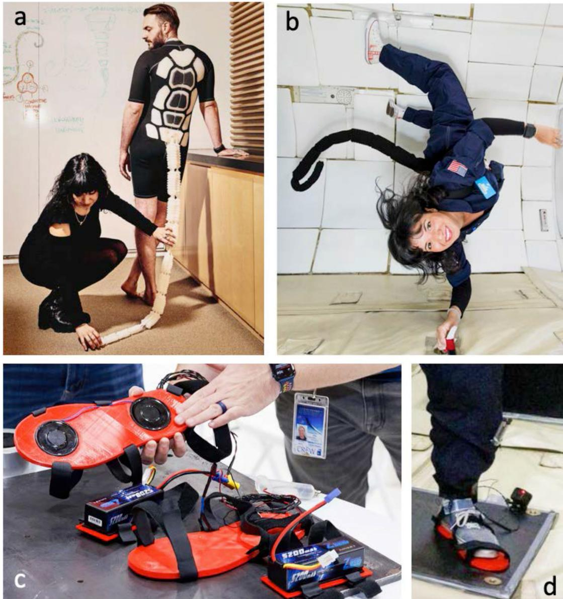
**FIGURE 2.** Dynamic astronaut restraint systems: SpaceHuman (a) tail linkage skeleton, (b) deployed with active pneumatics during 0-G test flight; and active magnetic outsole, (c) in prep, and (d) during 0-G Test Flight.
