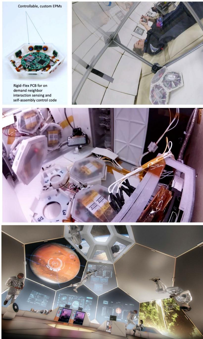
**FIGURE 4.** TESSARAE test tile, circuitry (top left) and in active deployment on a 0-G flight (top right); and on the International Space Station (middle); conceptual view (bottom) of the interior of an assembled structure depicting several Space Initiative projects, including some described here, in action.
