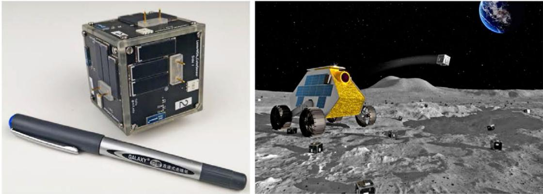
**FIGURE 5.** Lunar wireless sensor node, working prototype (left) and conceptual ballistic deployment from a rover (right).
