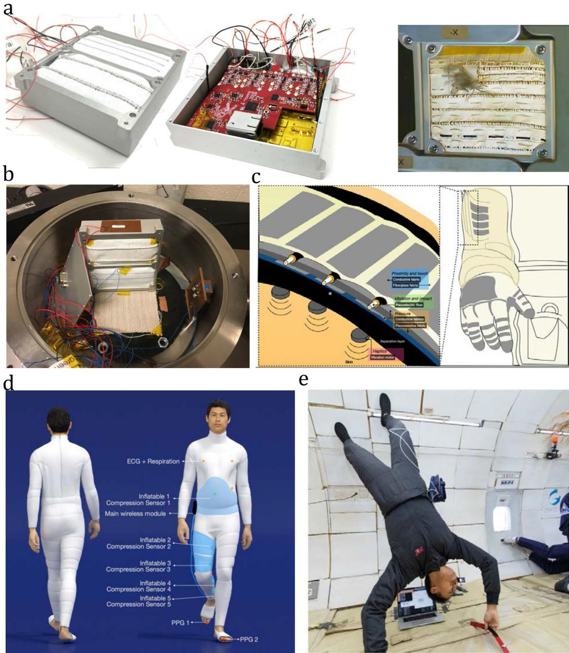
**FIGURE 1.** Smart textiles for space. (a) SpaceSkin with electronics (left/center) and passive sample flying outside the Space Station [right], (b) under TVAC Test, and (c) conceptual layout for SpaceSkin strips with opposing tactile actuators for the “Sensory Conductor” in a spacesuit arm. Peristaltic Suit layout (d) and working prototype during 0-G test flight.
