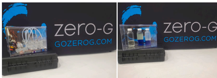
Fig. 3. Left - Top-choice experiment selected by astronaut Jeff Hoffman – acetic acid mixing with baking soda to produce CO 2 . Right - Second-choice experiment selected by astronaut Jeff Hoffman – mixing of oil and water.
