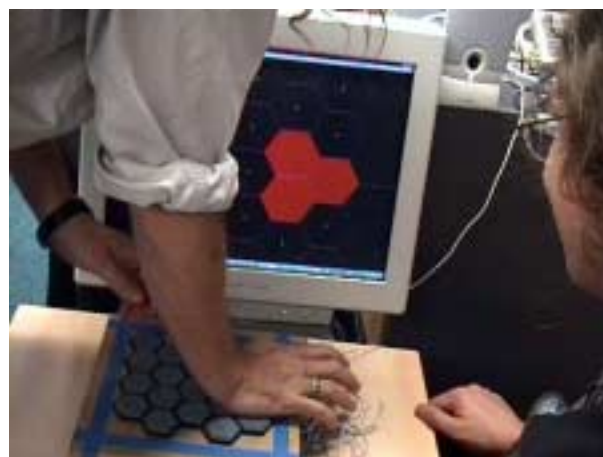
Fig. 1.3. The tile as a control device controlling a MIDI module, i.e. as a musical controller.
