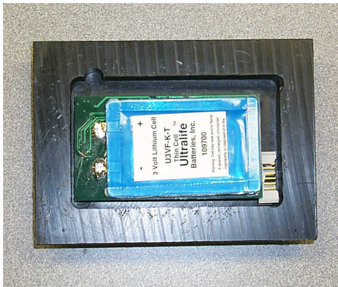
Photo 5: Node Circuit Board Inside Enclosure
