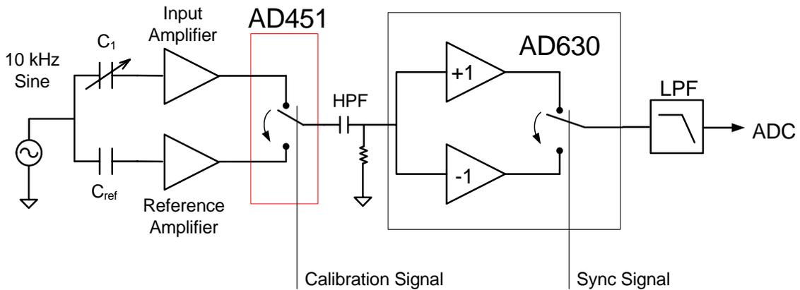
**Figure 16: Switched calibration circuit**
