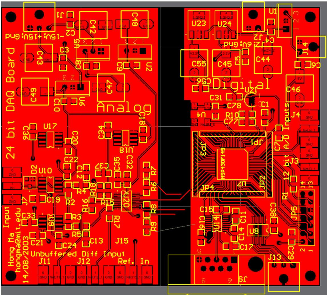
Figure 42: Data acquisition PCB layout, top layer
