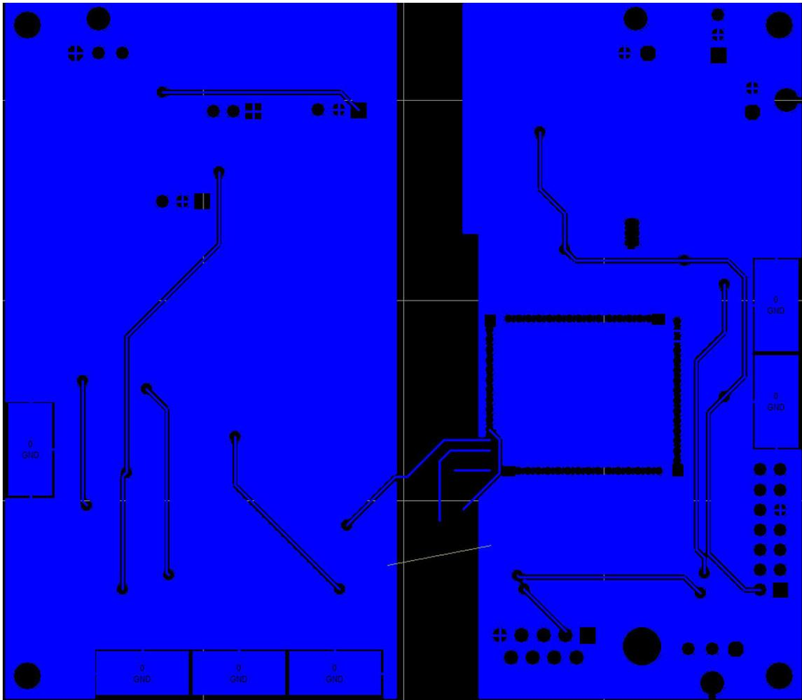
Figure 43: Data acquisition PCB layout, bottom layer
