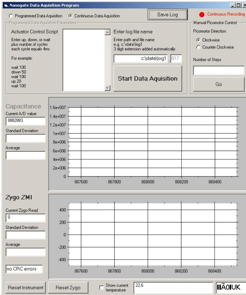
**Figure 18: Screen-shot of the Visual Basic data collection and user interface program**
