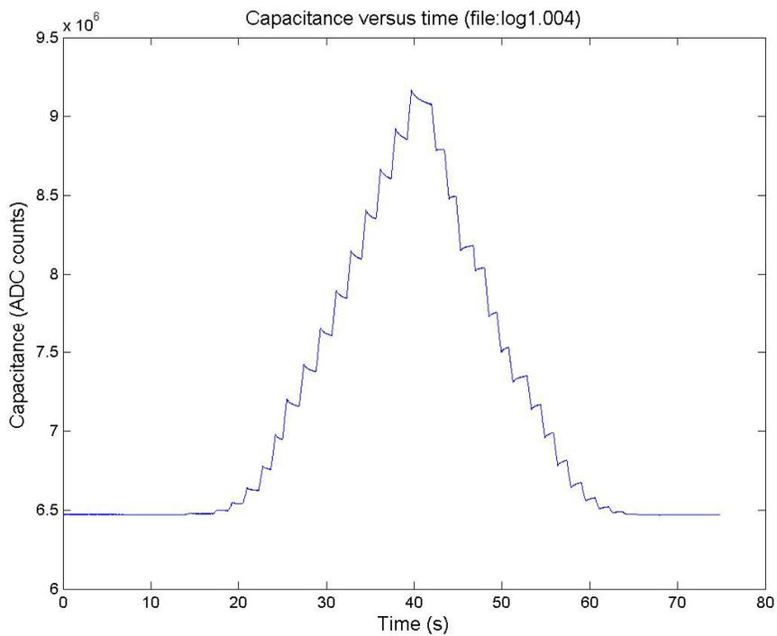
**Figure 23: Capacitance output in ADC counts versus time**
