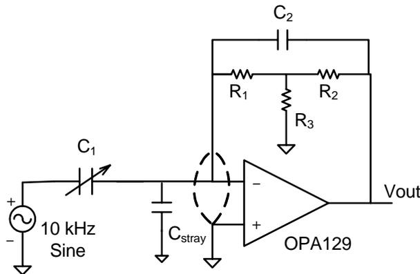
**Figure 14: Input Amplifier Schematic**
