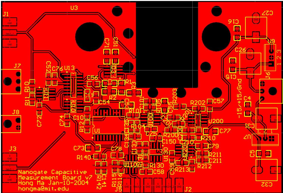
Figure 40: Analog front-end PCB layout, top layer
