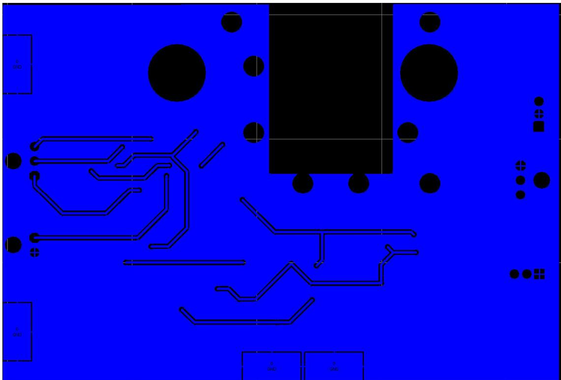
Figure 41: Analog front-end PCB layout, bottom layer
