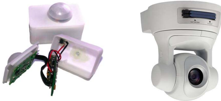
Figure 2.1 Left: a MERL motion detector node [8]. Right: the pan-tilt-zoom camera system the MERL team used to compare with the motion detection system.
