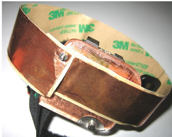
Figure 6-1: Bracelet electrode for capacitive sensor.
