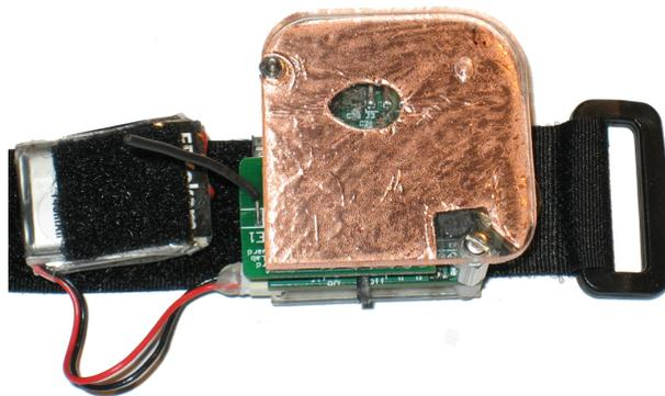
Figure 6-2: Faceplate electrode for capacitive sensor.
