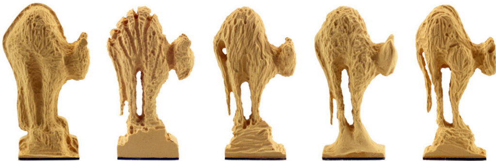
Figure 2.20 Five cats made by five participants using the FreeD, all using the same CAD model.
