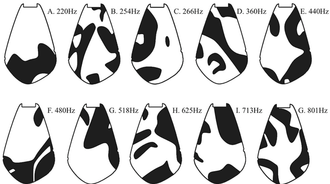
Figure 3.14: Eigenmode gradient maximum values. For each mode, the black areas are sensor locations candidates – the one third of the surface area with the highest absolute value of gradient.
