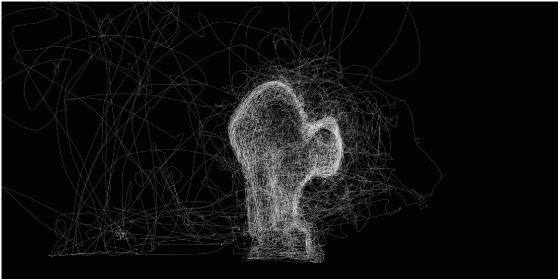
Figure 2.31 Tool-path visualization of Peter's work, documenting the whole carving process.
