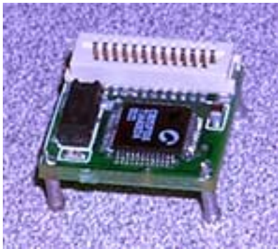
Figure 2-15: Pushpin Processing Module, based on the Cygnal C8051016 8-bit 8051-core microprocessor.
