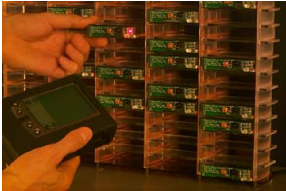
Figure 2-6: Media Matrix physical database. Each mini DV is tagged with a microcontroller capable of communicating with its neighbors, allowing for a user query entered wirelessly from a PDA to be passed from one tag to the next until it is satisfied.
