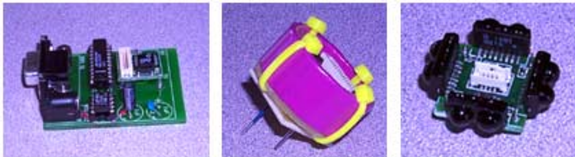
Figure 2-12: RS232 serial communication module with attached processing module (left), capacitive coupling communication module (purple antenna) with attached processing module and power module (center), and IR communication module (right).
