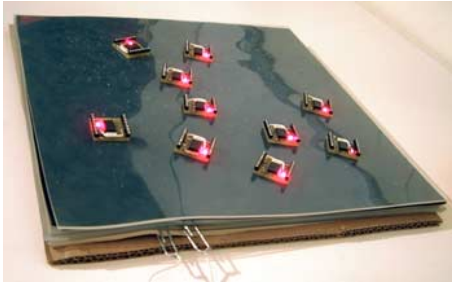
Figure 2-4: Initial PIC-based 3-prong Pushpins embedded in a seven-layer substrate (power layer, ground layer, resistive communication layer, and intervening insulating layers). Each prong electrically contacts a different layer to provide the Pushpin with power and a communication channel.
