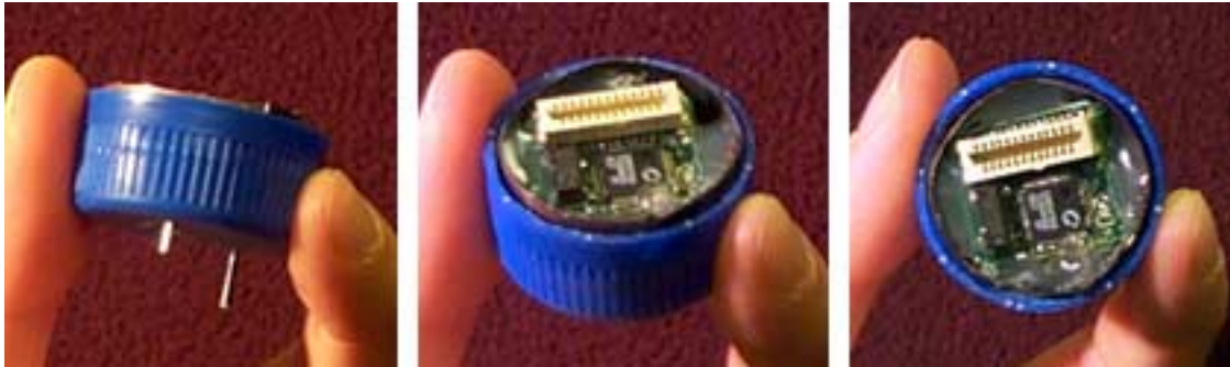
Figure 2-14: An early prototype of the capacitive coupling-based Pushpin was housed in a bottle cap. A copper antenna lines the inside of the bottle cap, encircling the processing module.
