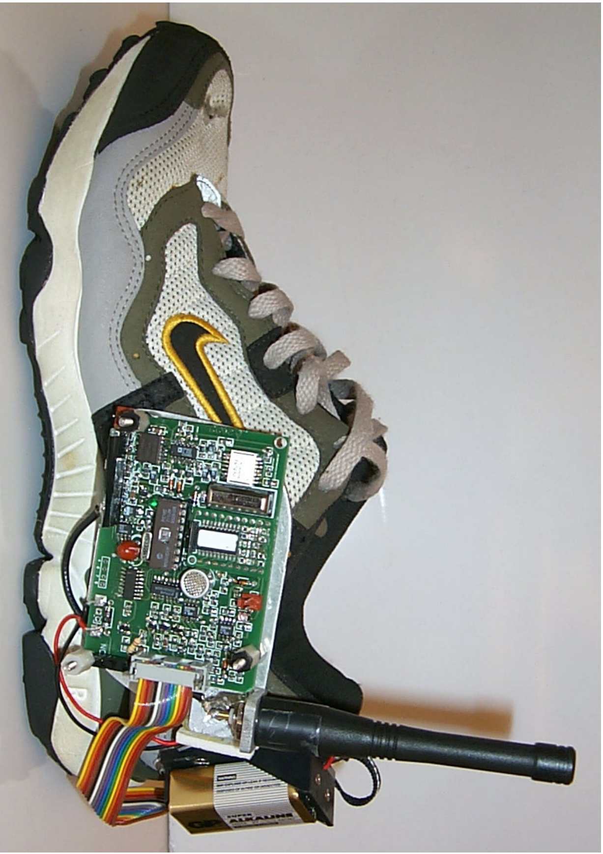
Photo 3: The Expressive Footwear - 16 diverse sensor channels wirelessly transmit from the foot of a performer for producing dance-driven interactive music
