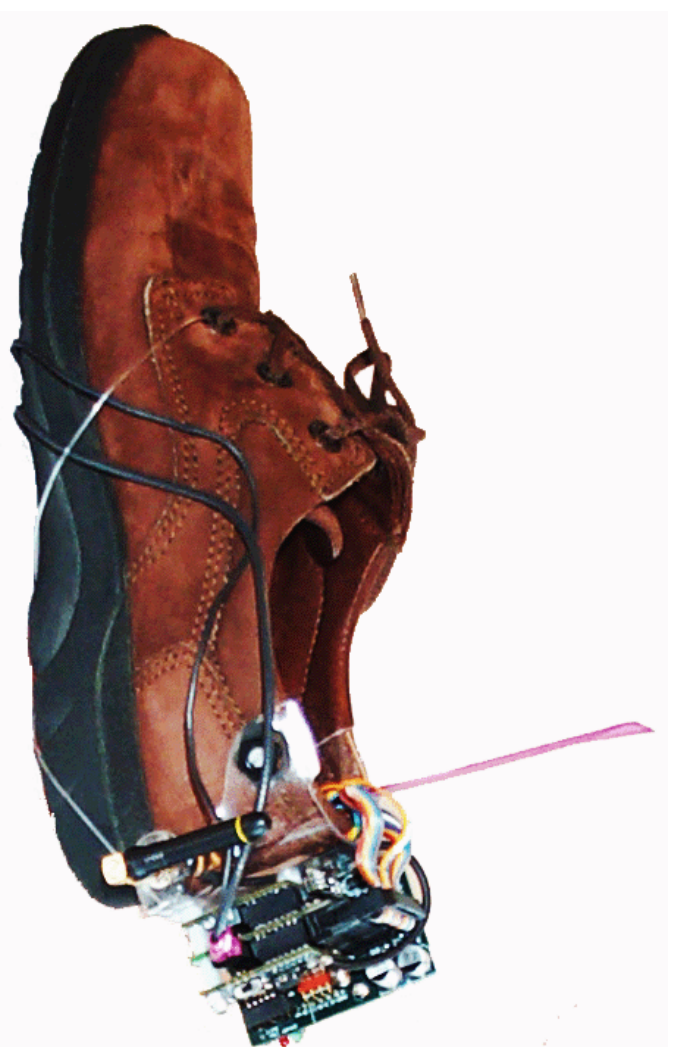
Photo 4: The Stack Sensor Architecture - a compact, configurable, multimodal wireless sensing platform (top) and its application in a shoe to monitor gait characteristics (bottom)
