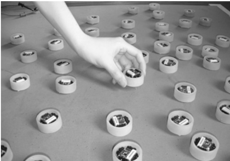
Fig. 3. Pushpins equipped with IR communication modules (and white diffuser rings) drawing power from the laminate substrate
